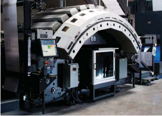
The arched paper path is critical for stabilising paper moving through the print zone because it reduces wet cockle effects and controls printhead to paper spacing.
