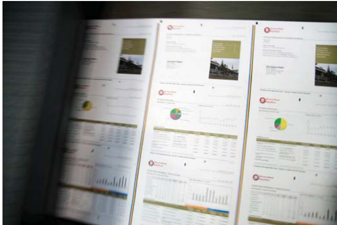
Across its 762mm width the IWP can print 2600 US Letter (8.5 x 11ins) pages per minute with a throughput of 400ft (122 metres) per minute of stocks up to 200 gsm.
