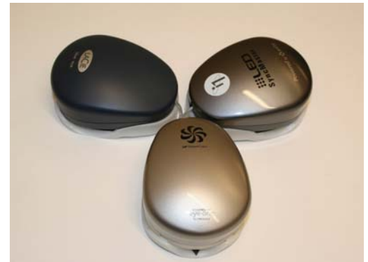
By far the most popular measuring device for vendors to bundle with a high-end proofing monitor is the X-Rite Display 2 colorimeter.
